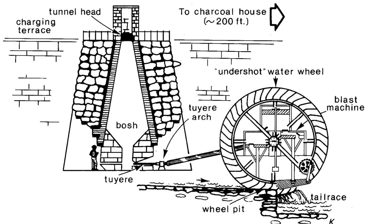
**Figure 103.** Generalized illustration of a typical 19<sup>th</sup> century iron furnace. From Inners (1986, fig. 4).
