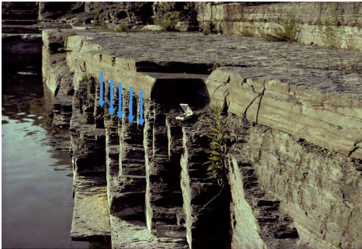
Figure 6-3. J 2 joints in the Ithaca Formation at Taughannock Falls State Park where multiple en-echelon cracks propagate down into shale from a siltstone-shale interface.
