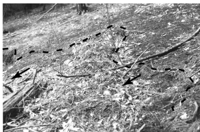
Figure 77. Irregular tension cracks (below dashed line) several inches high and a few tens of feet northeast of the initial failure area. Arrows show slight downward movement of the soil.
