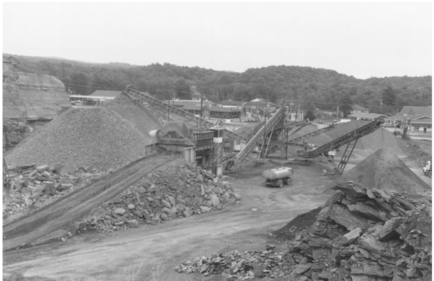
Figure 36. Operations at Riccobono's quarry, showing the various crushers and numerous piles of processed stone. The primary crusher is in the center of the photo.
