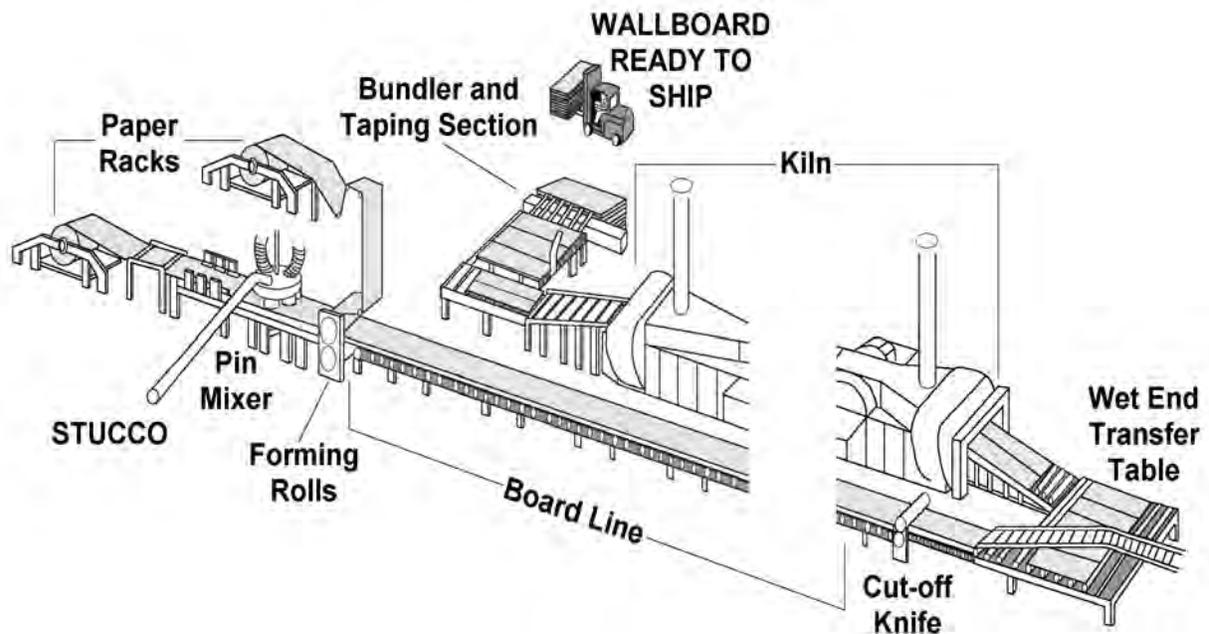
**Figure 88.** Schematic diagram of National Gypsum Company's gypsum wallboard manufacturing process
