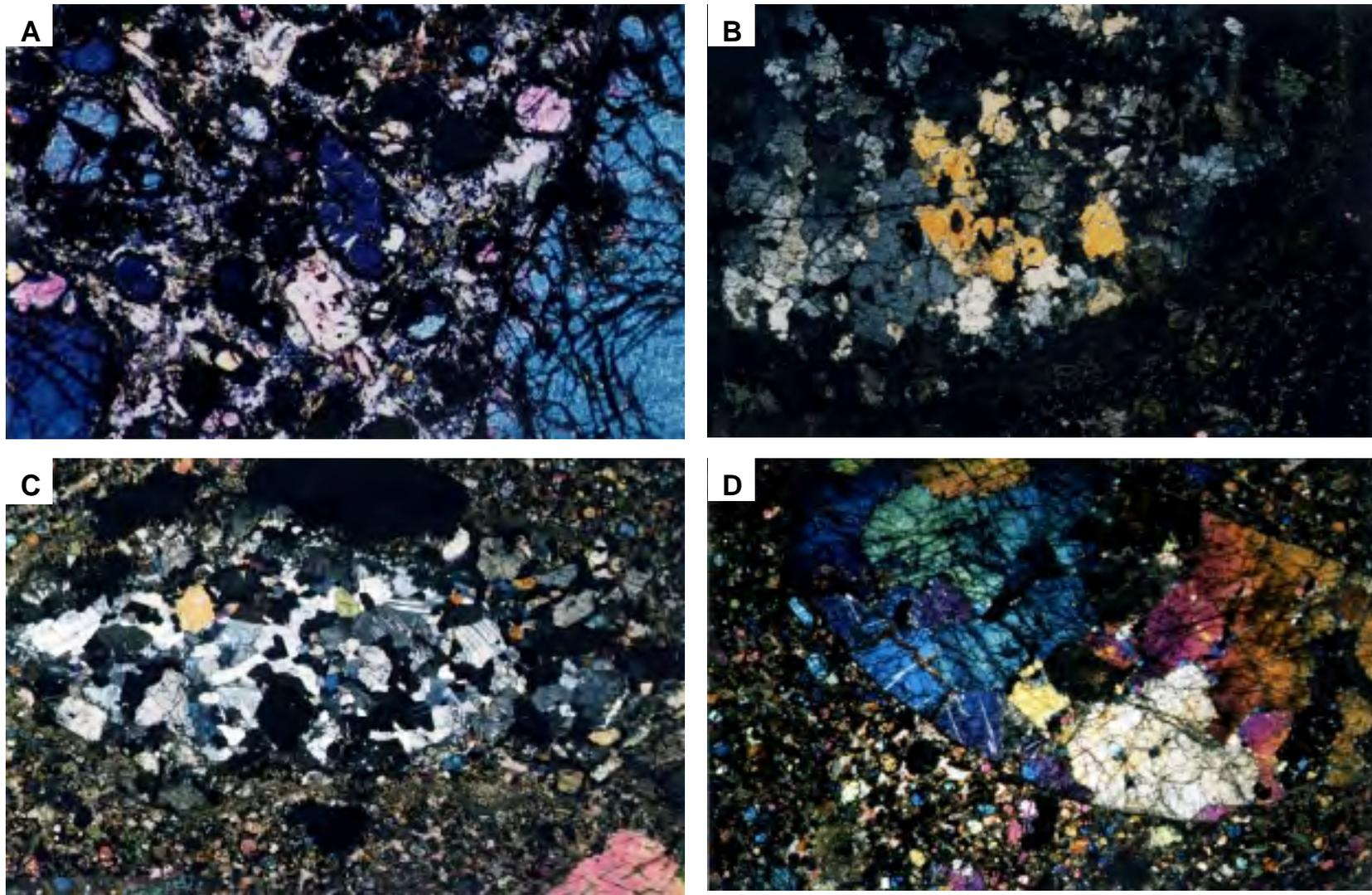
**Figure 35.** Photomicrographs of the Masontown Kimberlite, all under cross polarizers. A. Unaltered kimberlite. Field of view = 4 mm. B. Granitic gneiss xenolith in the kimberlite. Xenolith is 0.8 in (2 cm) long, and the quartz grains have an anomalous yellow color due to an overly thick slide. Field of view = 4 mm. C. Eclogite xenolith in kimberlite. Field of view = 4 mm. D. Spinel dunite xenolith in kimberlite. Field of view = 3 cm.
