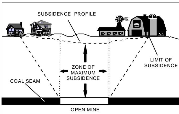
**Figure 14.** When a mine opening collapses, more surface area is affected than just the land directly above the collapsed void (modified from Pittsburgh Geological Society, 1999b). \*Angle of Influence – under much discussion and dispute, particularly for longwall mining.
