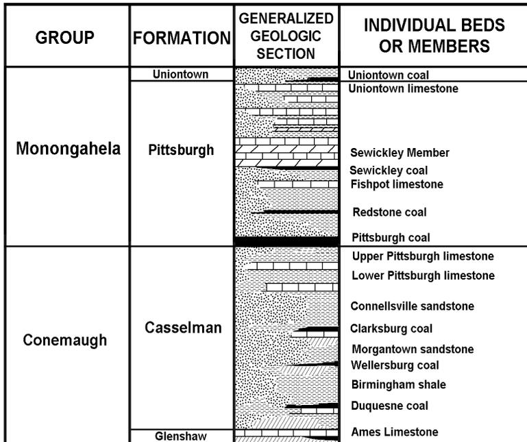
**Figure 44.** Generalized geologic column of the exposed rocks in the project area.
