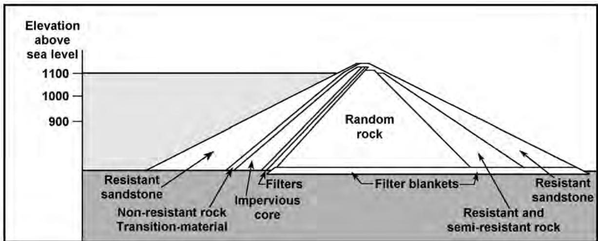
**Figure 82.** Cross sectional diagram of Little Blue Run Dam from south (left) to north (right). Modified from Ruppen and Briggs, 1995.
