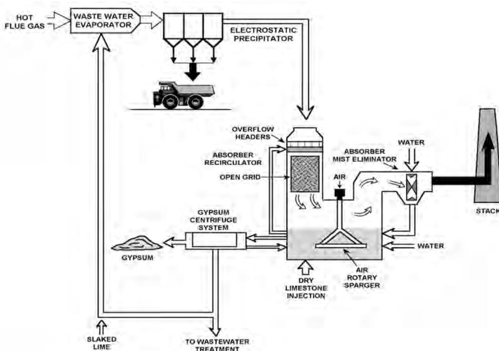
**Figure 87.** Schematic diagram of wet flue gas desulfurization (FGD) technology.
