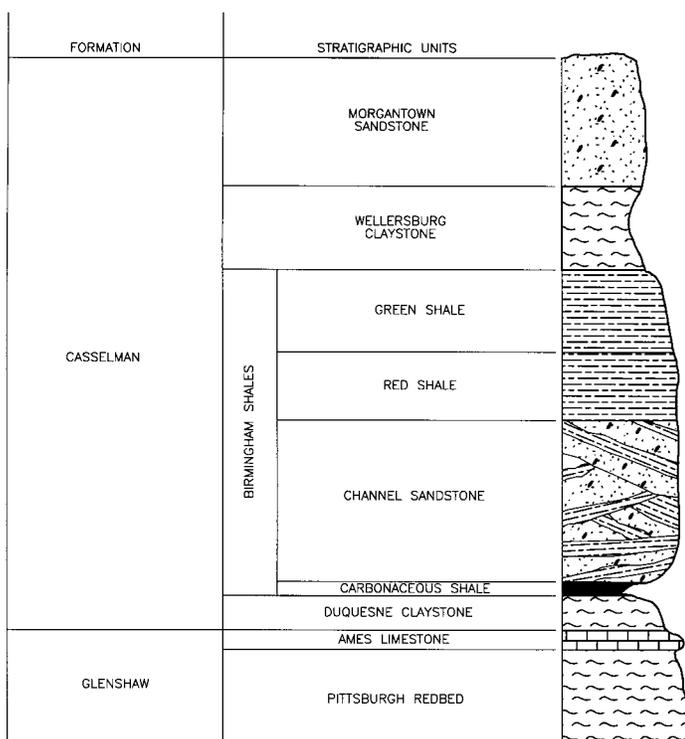
**Figure 56.** Generalized stratigraphic section illustrating the lithologic units of the Duquesne Bluff slope.
