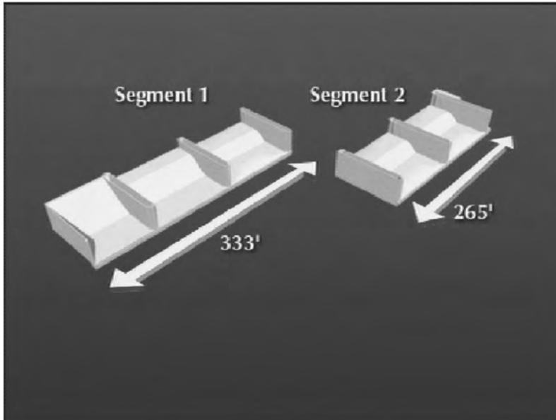
**Figure 50.** Dimensions of float-in dam segments.
