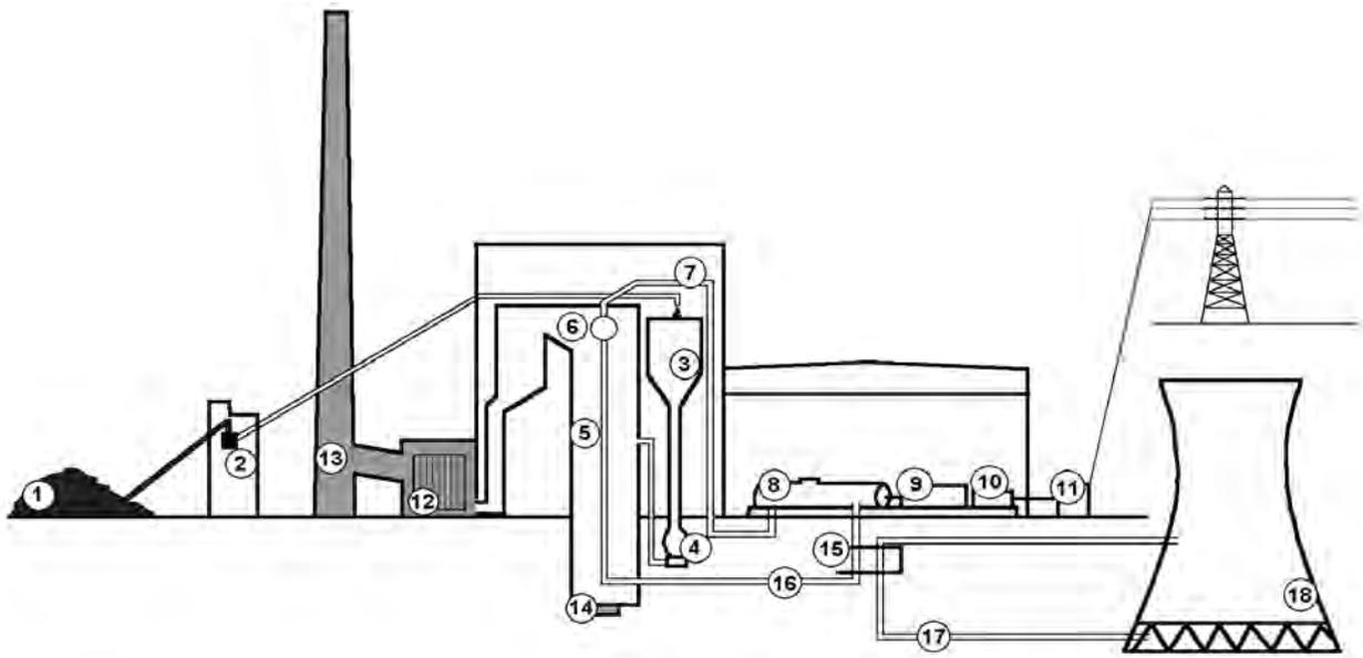
**Figure 86.** Schematic diagram of a coal-fired electrical generation plant. Numbered items are described in Table 8. The environmental controls are shaded.
