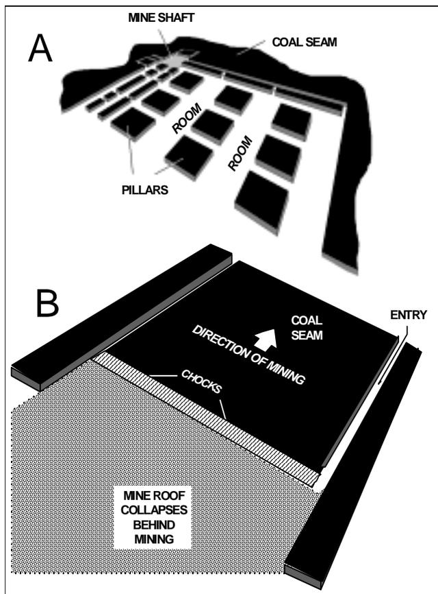
**Figure 13.** Diagrams of coal mining methods (from Pittsburgh Geological Society, 1999b). A. Room-and-pillar mining. Pillars of coal are left in place to prevent the mine roof from collapsing during mining. These are removed during retreat mining. B. Longwall mining, showing collapse of the mine roof as mining advances and the chocks are moved forward.
