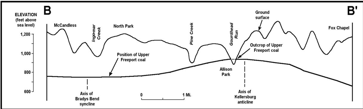
**Figure 6.** Cross section B-B' across the Bradys Bend syncline and Kellersburg anticline in northern Allegheny County (from Harper, 1995a). See Figure 5 for location.
