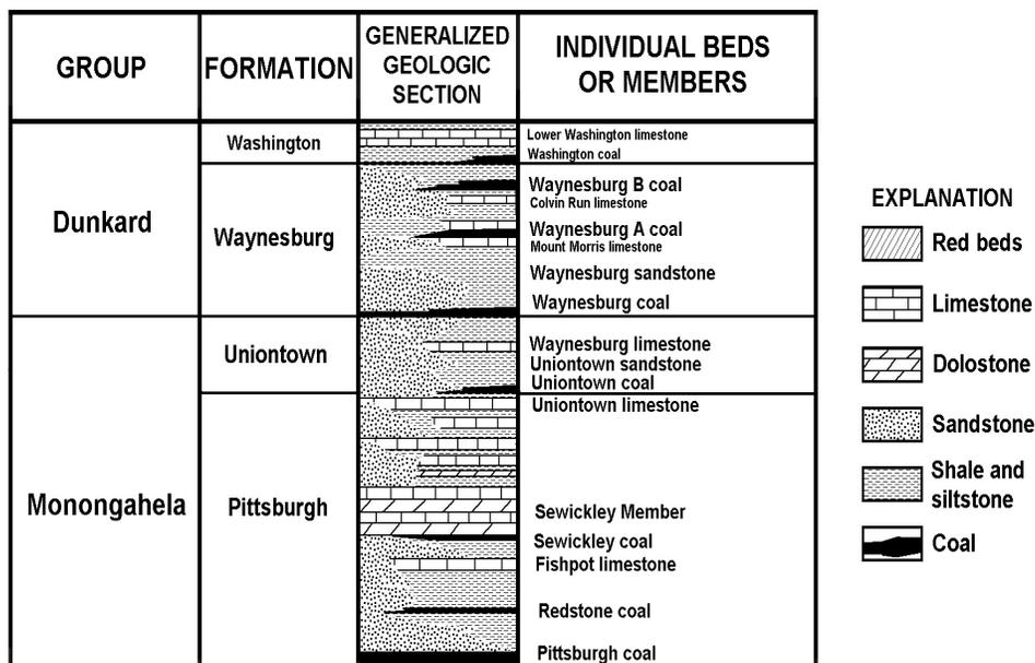
**Figure 33.** Generalized geologic column of the country rock exposed in the area of the Masontown kimberlite dike.
