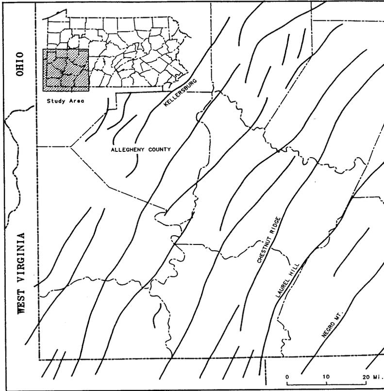
**Figure 4.** Map of southwestern Pennsylvania showing the trends of the major anticlinal axes. The three most prominent, Chestnut Ridge, Laurel Hill, and Negro Mountain anticlines, form high, deeply dissected ridges. From Harper (1995a).
