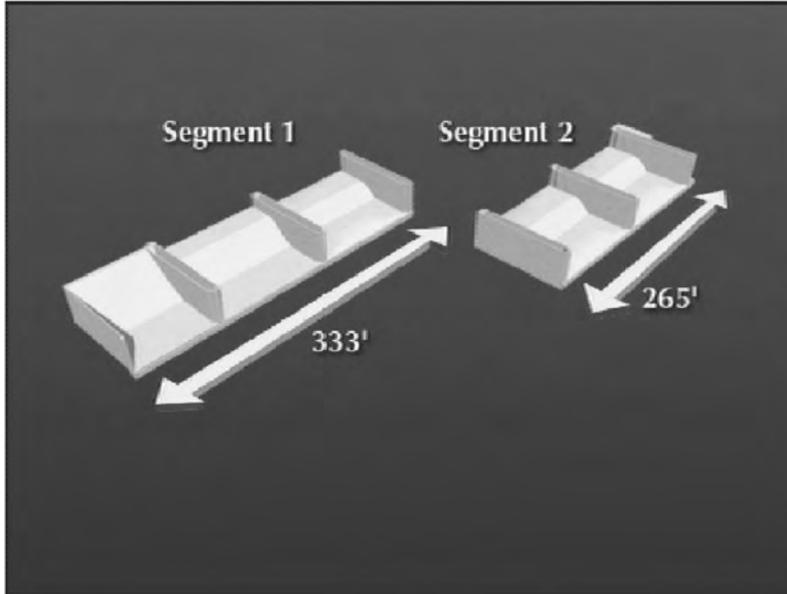
**Figure 50.** Dimensions of float-in dam segments.
