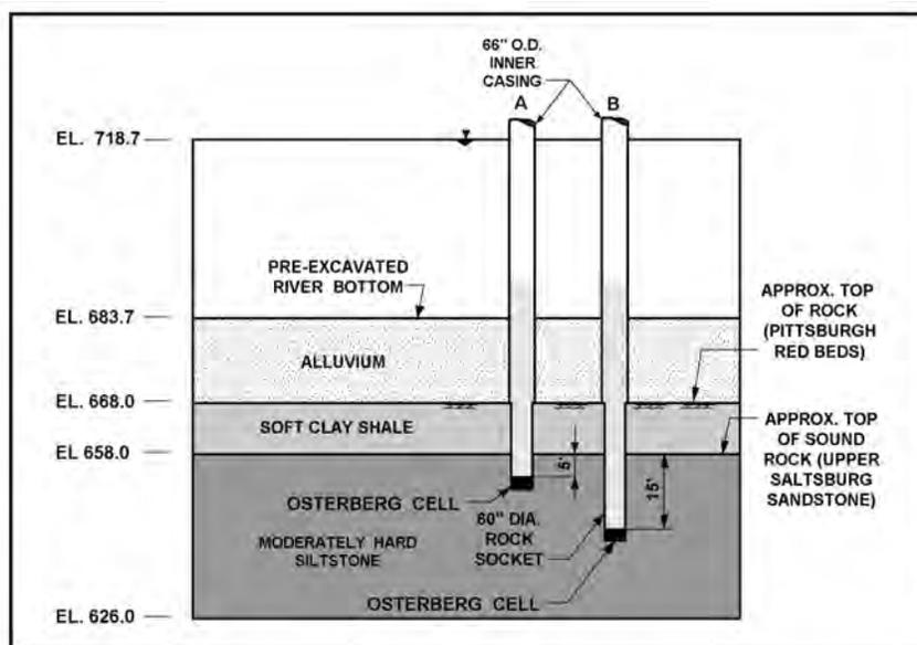
**Figure 48.** Geologic cross section of the new Braddock dam project site with test drilled shafts.
