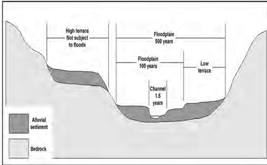
**Figure 20.** Cross section of a typical western Pennsylvania river valley showing the extent of flooding from periodic (1.5-year), 100-year, and 500-year floods. High terraces, formed before and during the Pleistocene, commonly occur between 150 and 250 feet above current river levels (from Pittsburgh Geological Society, 1999c).
