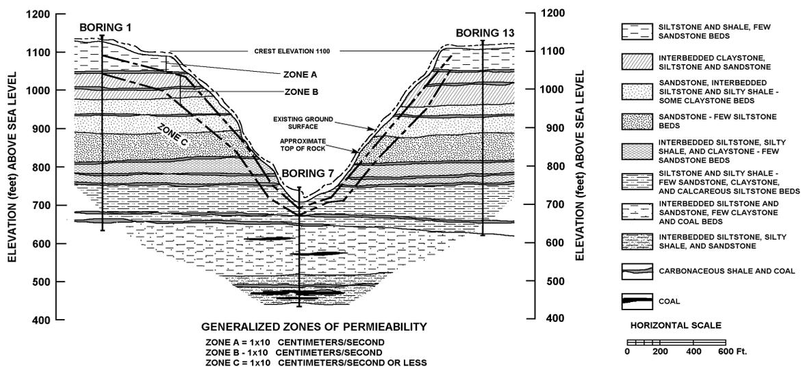
**Figure 83.** Generalized geologic cross section of the Little Blue Run valley (modified from Thiers and others, 1976).
