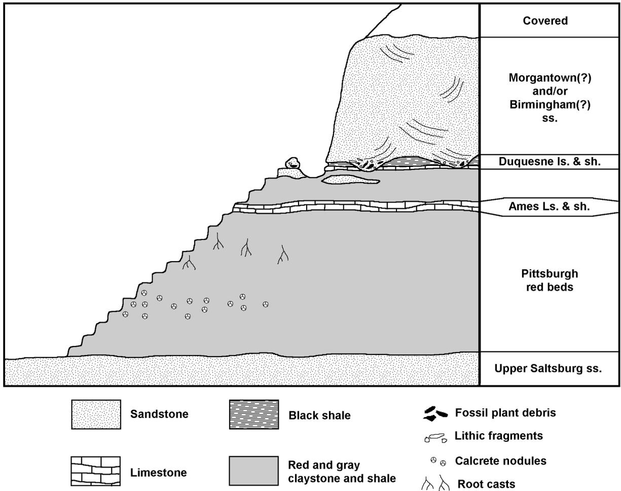
**Figure 28.** Generalized topographic and stratigraphic cross section of the “I-279 Fossil Collecting Locality” roadcut (from Shultz and others, 1995).
