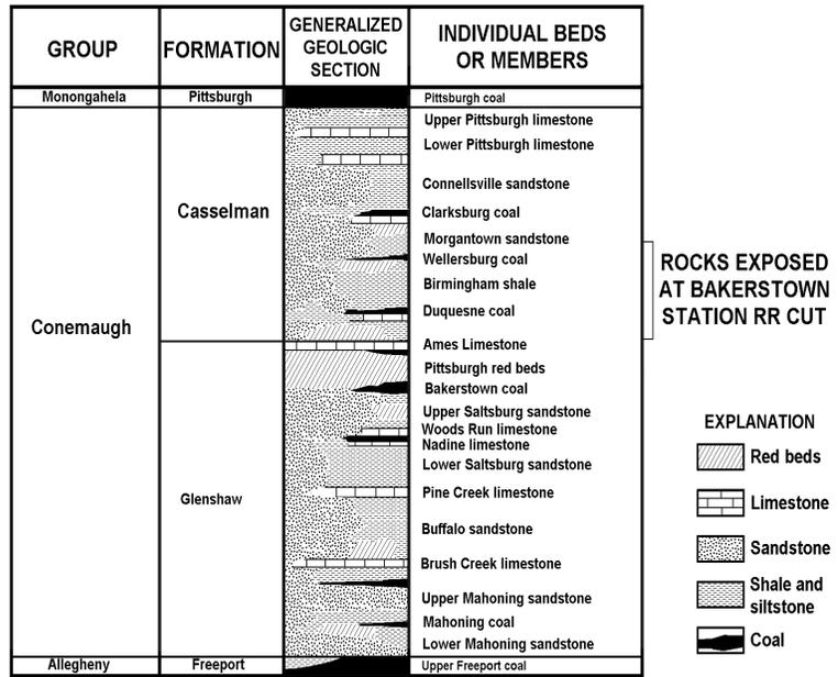
**Figure 74.** Generalized geologic column of the exposed rocks in the Bakerstown Station railroad cut.
