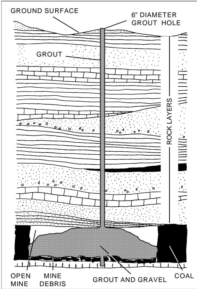
**Figure 16.** Using a grout column to fill a mine void (from Pittsburgh Geological Society 1999b).
