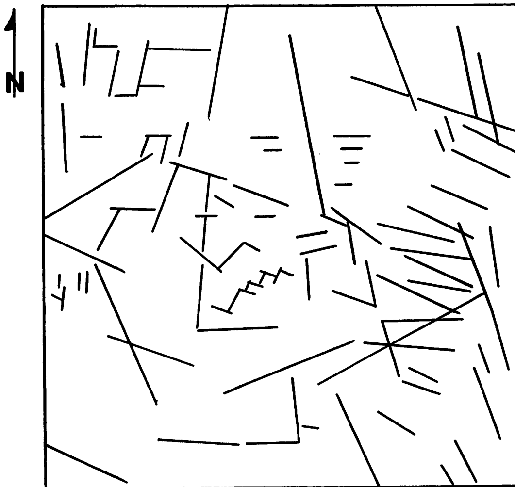
Figure 14. Lineament map of Cambria County and vicinity showing the traces of the interpreted linear features from a topoimage (Figure 13), second derivative Bouguer gravity, and second derivative magnetic intensity maps, all at 1:500,000 scale.
