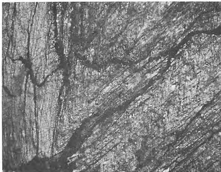
Figure 33. Photomicrograph showing cone-in-cone and stylolite structures in a carbonate layer at the top of the Riddlesburg Shale
