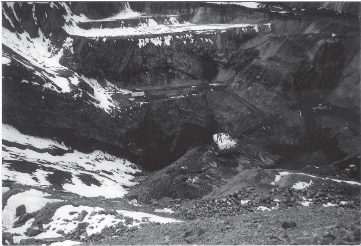
Figure 3-10. Coal Ridge synclinal axis at loader, and a Marion 7400 dragline mining the southern syncline. Thrust faults are evident at the top of the photo, with an imbricate thrust visible. Looking west.
