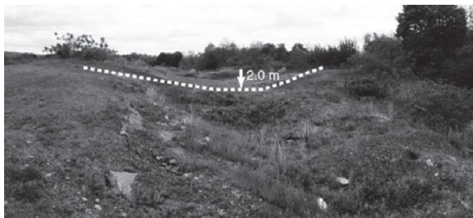
Figure 1-7. Example of recent subsidence near Ss. Peter & Paul Cemetery. This sinkhole began to form in 2011. (Photo: Elick 2015)
