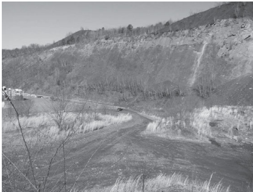
Figure 11-11. Steeply inclined highwall exposing the seatrock of the Mammoth Bottom Split (No. 8) at 1. On top of Mine Hill in the background are old culm banks of the St. Clair Coal Co. Colliery.
